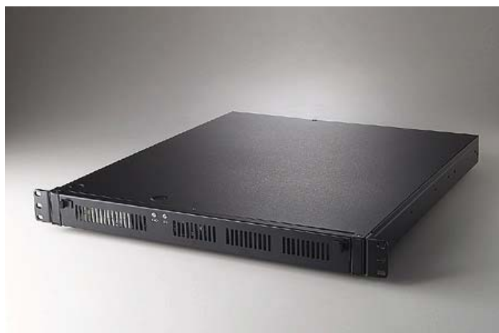
The S2 Enterprise (shown) and S2 Enterprise Ultra fit standard 19" racks
